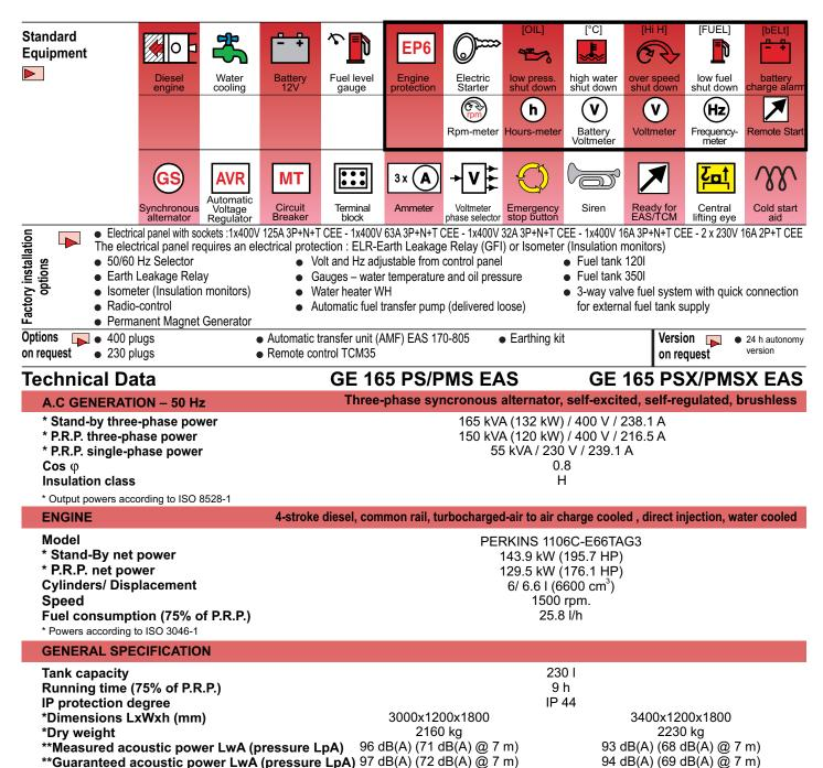
\* Dimensions and weight without trolley/trailer. \*\*Acoustic power according to European Directive 2000/14/EC
